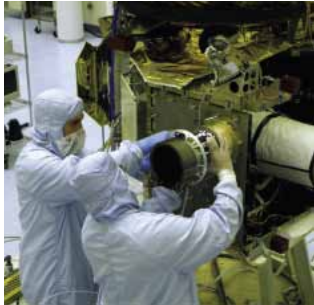
PLUTO-BOUND EXPERIMENT Technicians install the SWAP (Solar Wind Around Pluto) instrument, one of seven science packages carried by the New Horizons spacecraft.
