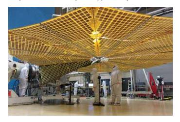
▲ CATCHIN' SOME RAYS Engineers check one of Lucy's solar arrays, which will power the spacecraft as it flies out to Jupiter's orbit. After launch, one array did not fully deploy; as of press time engineers were still assessing the problem but did not expect any effect on the mission.
