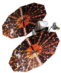
■ LUCY SPACECRAFT Lucy stretches more than 14 meters (46 feet) from tip to tip, thanks to its 7-meter-wide, decagonal solar panels.
